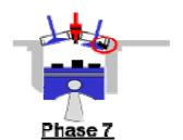
..and clamp between the annular valve seat and the exhaust valve Final Result: no compression, the engine does not start
