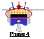
Combustion chamber with a small amount of deposits on the pitatop top Fuel residues caused by short drive cycles at low speecs starts accumulating in the combustion chamber
